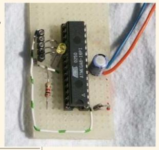
1 x ATmega8 DIP version, Atmel 8 bit Avr risc processor.
